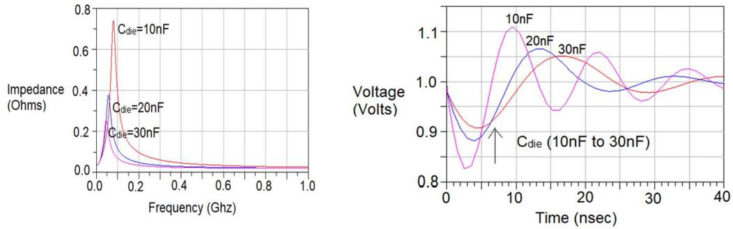
Figure2: PDN frequency response and transient response (for different ODC values)
