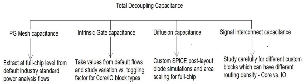
Figure 14: Post-layout ODC extraction flow
