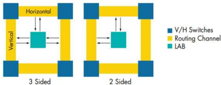
Figure 11: 2-side and 3-sided routing architecture ([8])
