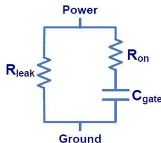
Figure 9: First order RC model for a logic circuit at certain operating state
