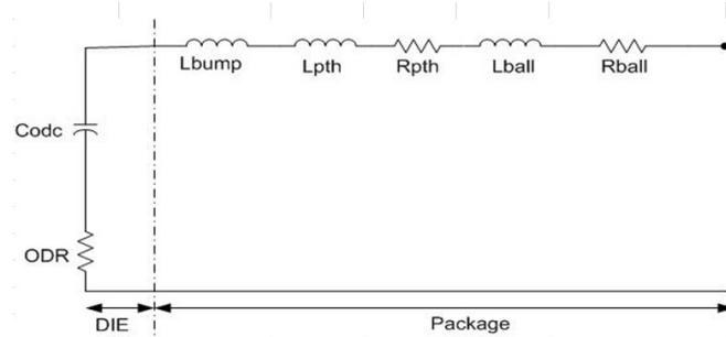
Figure 12: PDN model topology used to extract ODC from measured VNA data
