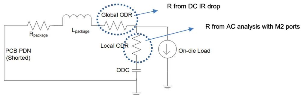
Figure 15: Representative lumped PDN model (showing local and global ODR)
