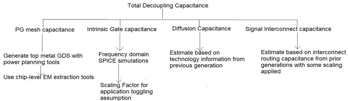
Figure 13: Pre-layout ODC extraction flow
