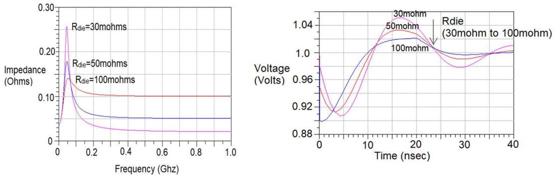
Figure 3: PDN frequency response and transient response (for different local ODR values)
