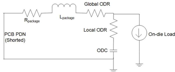
Figure 1: Representative System PDN Lumped model
