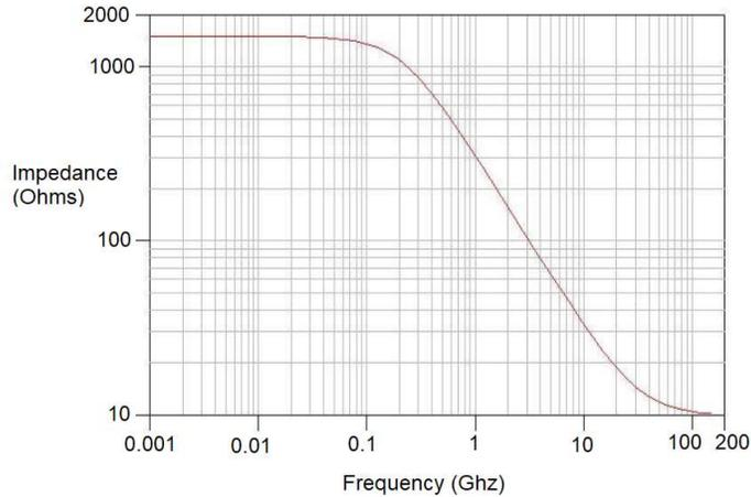
Figure 10:  $Z_{11}$  for a FPGA LE block when  $R_{leak}=1500\text{ohms}$ ,  $R_{on}=10\text{ohms}$  and  $C_{gate}=0.5\text{pF}$
