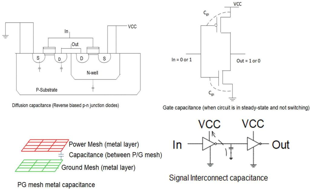
Figure 4: Sources of ODC in FPGA Applications
