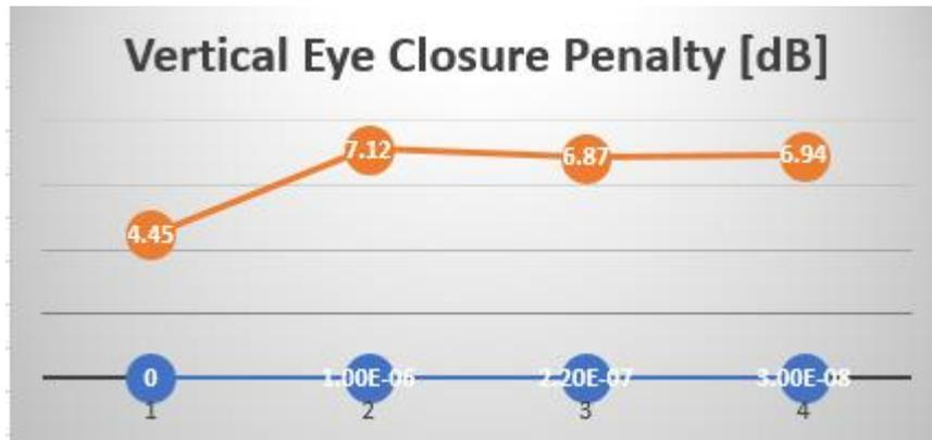
Figure 19 Vertical Eye Closure Penalty function of DC block.
