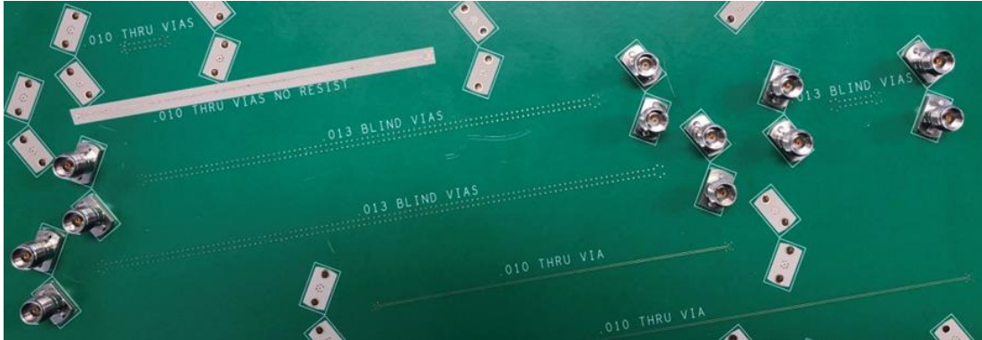
Figure 8 Photo of a portion of a Meg-4 RTF test platform courtesy of Ciena Corporation [18] used for model validation.
