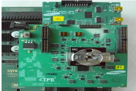
Figure 10: LPDDR5 Test Platform
