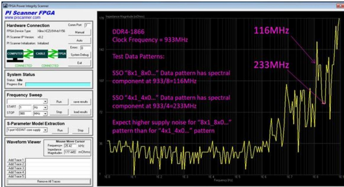
Figure 18. SSO data patterns having frequency spectral components aligned with a resonance peak and an impedance deep
