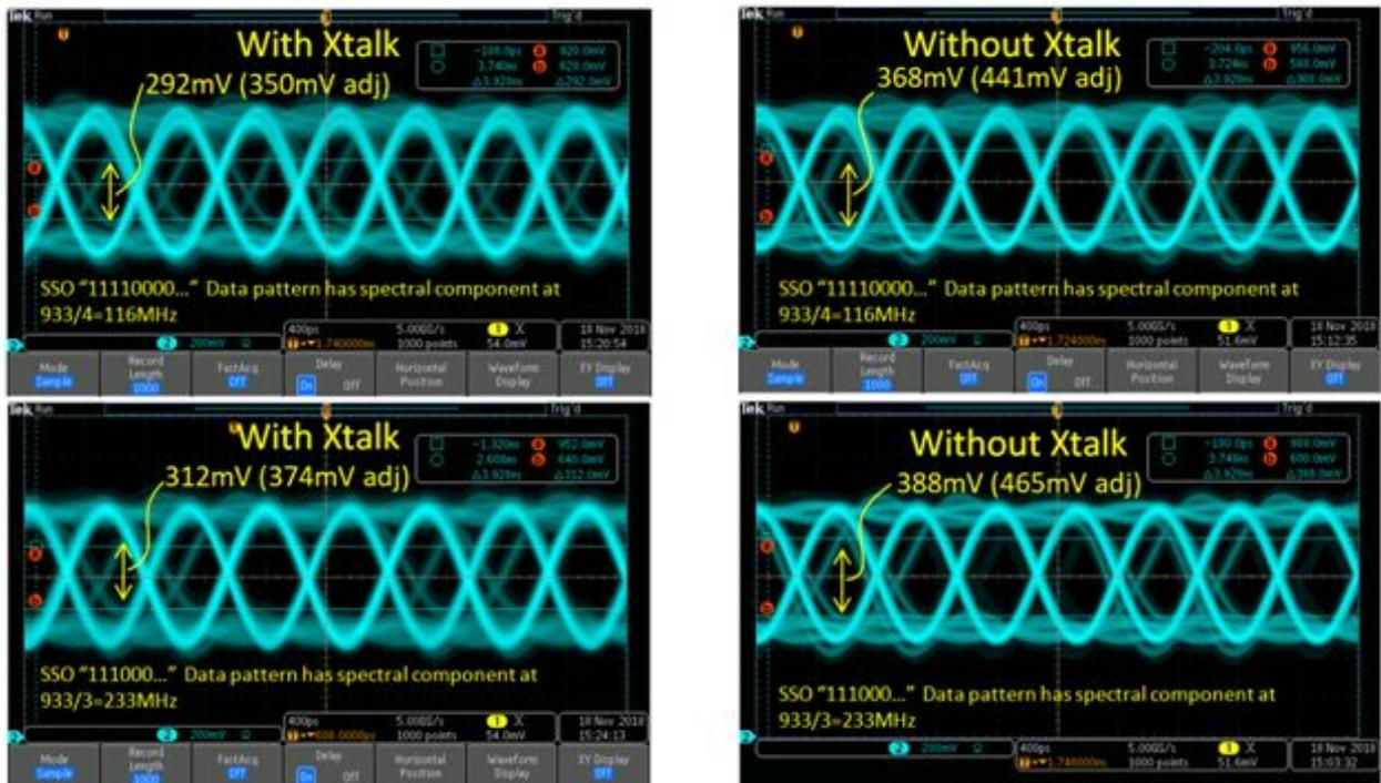
**Figure 22. DQ4 eye opening with and without crosstalk for the two SSO data patterns, “8x1\_8x0...” and “4x1\_4x0...”.**
