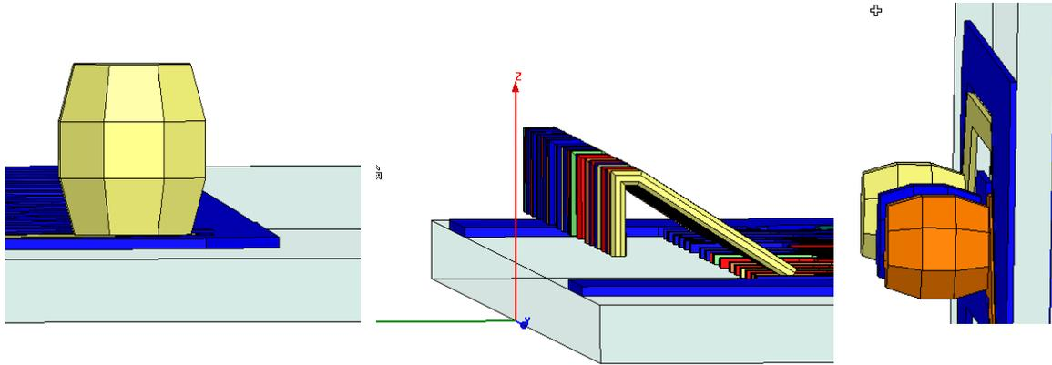
Figure 4 BGA balls and Bondwire modeling
