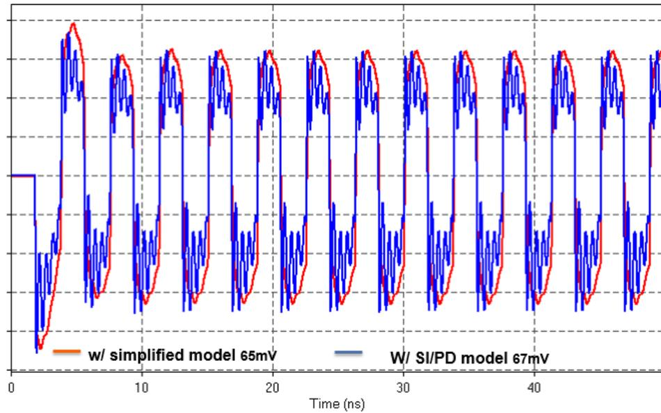
Figure 7 VddQ noise simulations at DRAM
