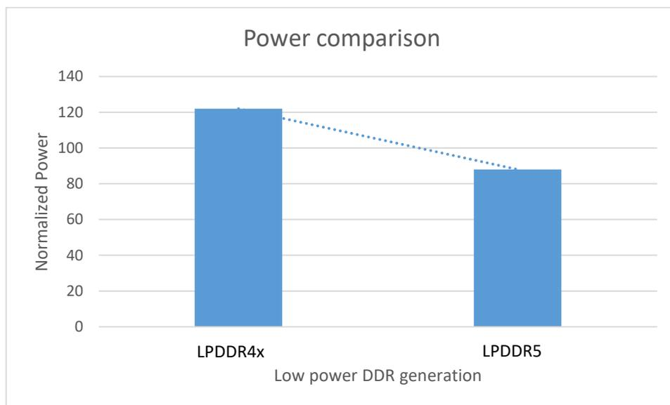
Figure 14. Performance comparison between LPDDR4x and LPDDR5
