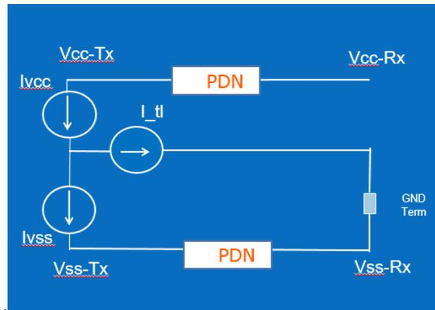
Figure 6 Final Stage Current for LPDDR
