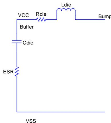
Figure 3 Equivalent PDN model for the LPDDR die
