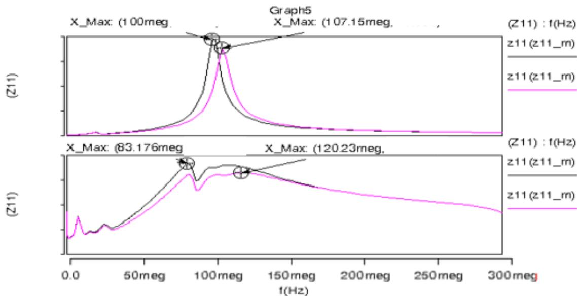
Figure 5 Self Impedance for VddQ and Vdd2 domains
