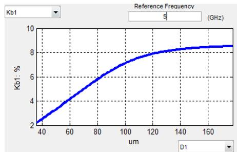
Figure-13 Dielectric thickness vs. Crosstalk Coefficient
