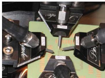
Figure 21. Step 2. Attach microprobes to the ends of the VNA cables
