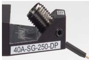
Thru connection, with the microprobe to be measured inserted, using unknown thru calibration
