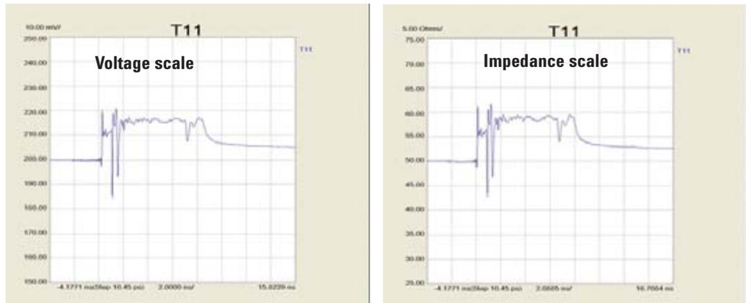
**Figure 9. T11 as reflected voltage and impedance profile.**
