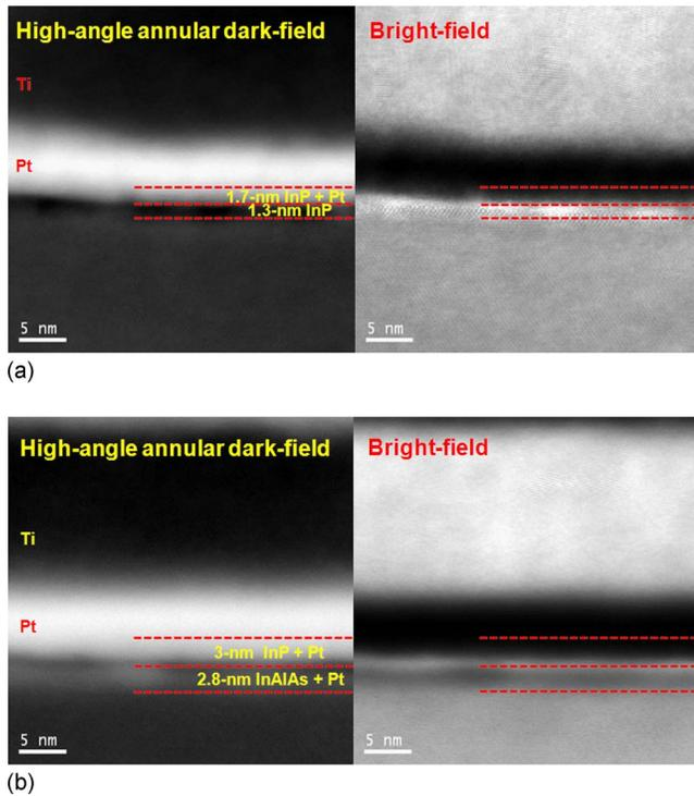
Fig. 2. (Color online) (a) Bright-field (left) and high-angle annular dark-field (right) STEM images of the Schottky contact fabricated on 3-nm-thick InP layer. (b) Bright-field (left) and high-angle annular dark-field (right) STEM images of the Schottky contact fabricated by utilizing buried-Pt technology on 3-nm-thick InP layer annealed at 325 °C.
