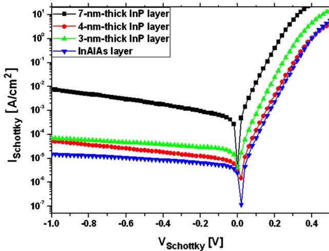
Fig. 4. (Color online)  $I$ - $V$  characteristic of the Schottky diodes fabricated on InP/InAlAs heterostructures having different InP layer thicknesses through a thermal annealing process at 350 °C.
