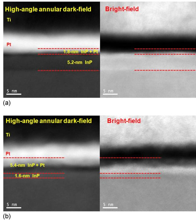
FIG. 1. (Color online) (a) Bright-field (left) and high-angle annular dark-field (right) STEM images of the Schottky contact fabricated on a 7-nm-thick InP layer. (b) Bright-field (left) and high-angle annular dark-field (right) STEM images of the Schottky contact fabricated utilizing buried-Pt technology on 7-nm-thick InP layer annealed at 325 °C.
