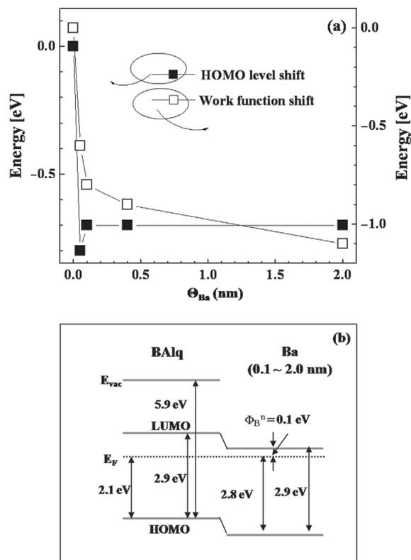
Fig. 3. (a) HOMO level shift [closed squares] of  $\text{HOMO}_{\text{BALq}} - \text{HOMO}_{\text{Ba-on-BALq}}$  and WF shift [open squares] of  $\Phi_{\text{BALq}} - \Phi_{\text{Ba-on-BALq}}$  as a function of  $\Theta_{\text{Ba}}$  on BALq at the pure BALq and Ba-on-BALq interface. (b) proposed energy band diagram for BALq and the Ba-on-BALq interface when  $\Theta_{\text{Ba}}$  between 0.2 and 2.0 nm is deposited on 10 nm-thick BALq.
