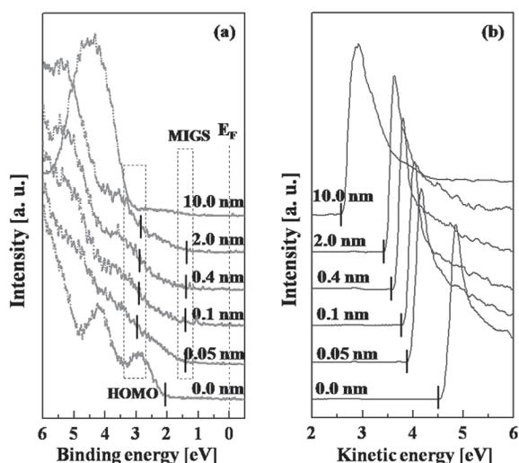
Fig. 2. UPS of the Ba-on-BALq interface. (a) spectral region around the BALq HOMO and (b) onset of photoemission with sample bias of  $-20$  V as a function of  $\Theta_{\text{Ba}}$ .
