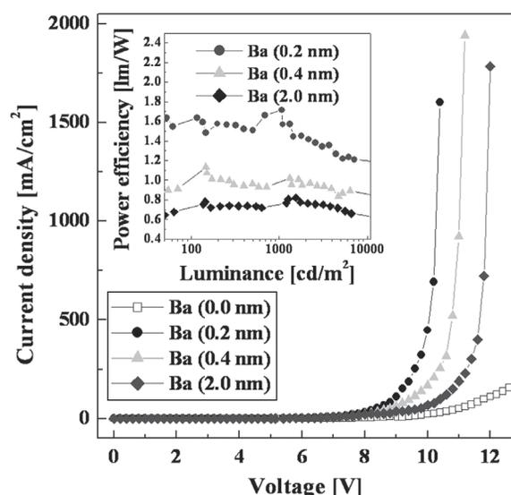
**Fig. 1.** Current density curves as a function of bias voltage. The inset shows the power efficiency–luminance curves. The devices were composed of glass/ITO/MoO<sub>3</sub> (5 nm)/2-TNATA (60 nm)/NPB (18 nm)/BAlq (22 nm)/Ba ( $x$  nm)/Al (100 nm). (Ba thickness of devices 0–3 = 0, 0.2, 0.4, and 2.0 nm, respectively).
