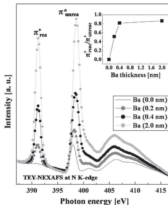
**Fig. 5.** TEY-NEXAFS spectra at the N K-edge of the Ba-on-BALq interface for the  $\Theta_{\text{Ba}}$  from 0 to 2.0 nm. The inset shows the intensity ratios for  $\pi_{\text{rea}}^*/\pi_{\text{unrea}}^*$  as a function of  $\Theta_{\text{Ba}}$  between 0 and 2.0 nm.
