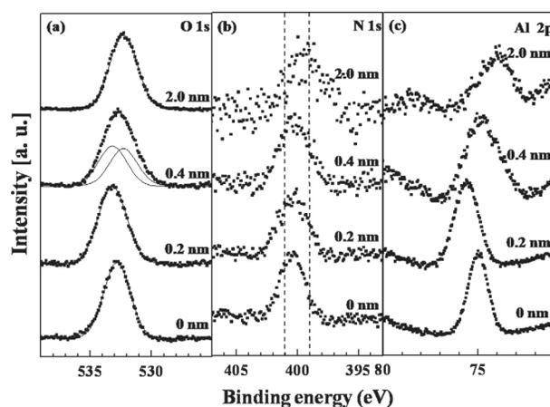
**Fig. 4.** Evolution of XPS O 1s (a), N 1s (b), and Al 2p (c) core level EDCs as a function of  $\Theta_{\text{Ba}}$  on BALq. The values in the figures indicate  $\Theta_{\text{Ba}}$ . The peak fitting of O 1s EDC was worked as Ref. [21].
