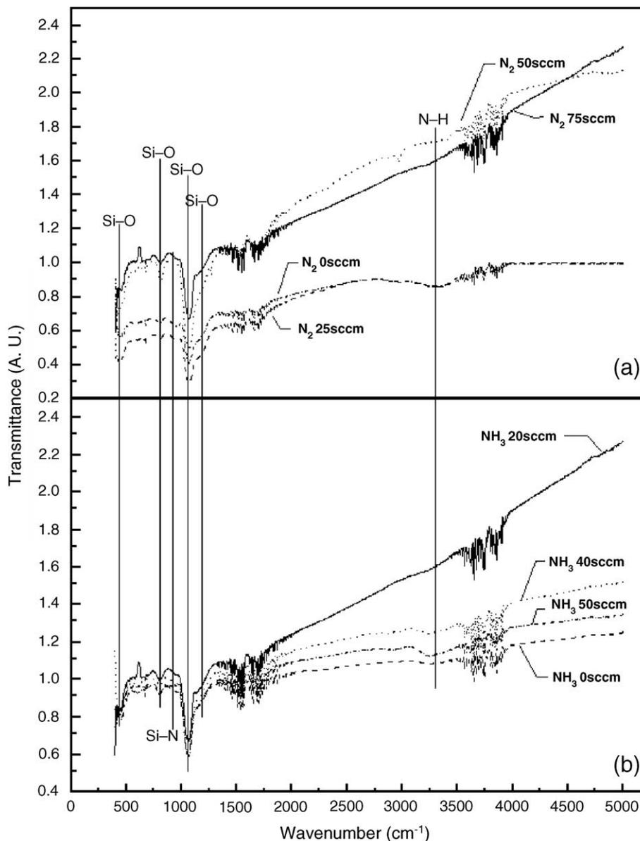
Fig. 3. FT-IR spectra of the  $\text{SiO}_x\text{N}_y$  deposited under different (a)  $\text{N}_2$  gas flow rate and (b)  $\text{NH}_3$  gas flow rate by the PECVD (process condition: TEOS 15 sccm,  $\text{O}_2$  flow rate 10 sccm, rf power 300 W, and dc bias voltage  $-150$  V). Also, when  $\text{NH}_3$  was varied,  $\text{N}_2$  flow rate was 75 sccm and, when  $\text{NH}_3$  flow rate was varied,  $\text{NH}_3$  flow rate was 20 sccm).
