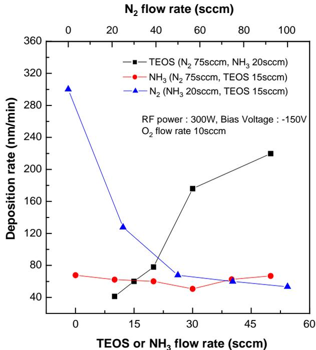
Fig. 2. Deposition rate of  $\text{SiO}_x\text{N}_y$  films as a function of TEOS flow rate;  $\text{NH}_3$  flow rate; and  $\text{N}_2$  flow rate at 300 W of the rf power and  $-150$  V dc bias voltage.
