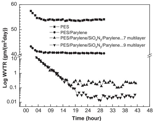
Fig. 4. WVTR of multilayer thin films composed of parylene (800 nm)/SiO<sub>x</sub>N<sub>y</sub> (60nm)/parylene (280 nm)/SiO<sub>x</sub>N<sub>y</sub> (600 nm)/... on 200 μm-thick PES.
