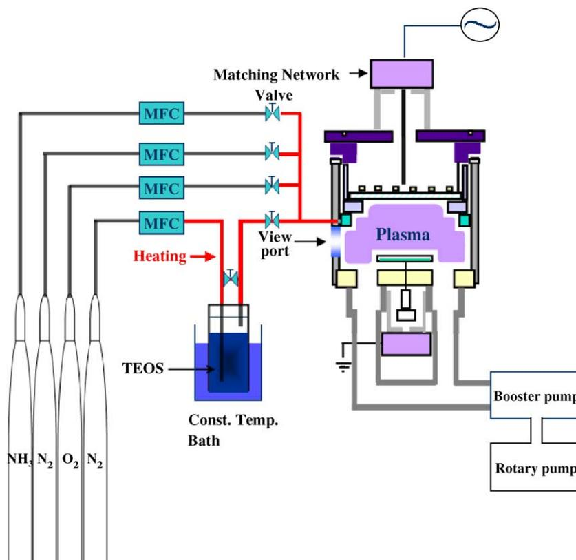
Fig. 1. Schematic illustration of an ICP-type PECVD apparatus with a bubbling system of TEOS used in this study.
