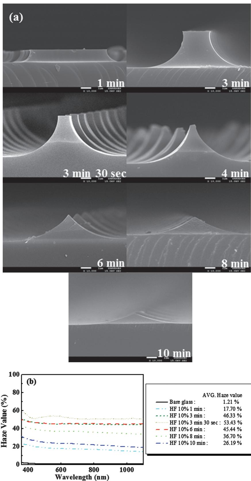
**Figure 2.** Characteristics of periodically textured glass substrate: (a) cross-sectional SEM image of textured glass substrate, and (b) haze values of textured glass substrate. It could be seen that the slopes were too steep when the etching time was not sufficient. Etching time of more than 6 min was required for stable *p*-layer deposition of the thin film solar cells.
