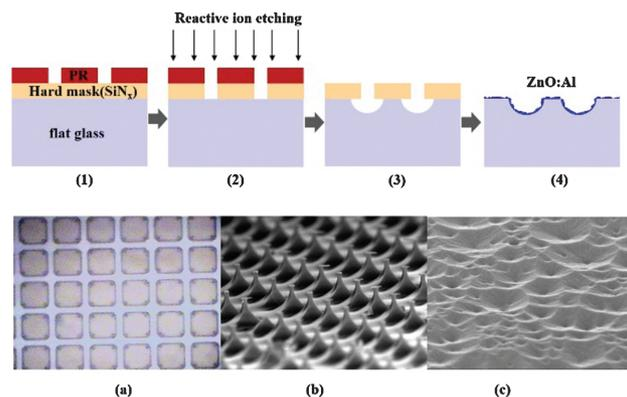
**Figure 1.** The first line (1–4) shows the process flow of the fabrication of doubly-textured substrate. The second line shows (a) an optical microscope image of the photoresist-patterned glass substrate, (b) an SEM image of the surface textured glass substrate, and (c) an SEM image of the etched ZnO:Al.
