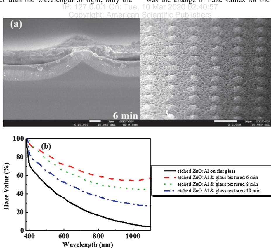
**Figure 3.** Characteristics of doubly-textured substrate: (a) SEM images of etched ZnO:Al on textured glass substrate, and (b) haze values of etched ZnO:Al on flat and textured glass.
