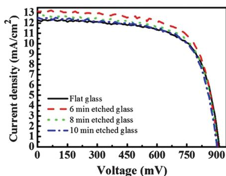
**Figure 4.** Current density versus voltage ( $J$ - $V$ ) characteristics of the a-Si:H thin film solar cells on doubly-textured substrates with different glass etching times.
