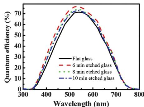
**Figure 5.** The Quantum Efficiency (QE) of a-Si:H thin film solar cells on doubly-textured substrate with different glass etching times.
