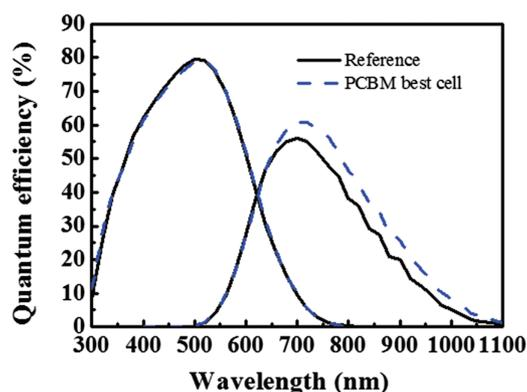
**Figure 5.** Quantum efficiency of reference and PCBM tandem cells.
