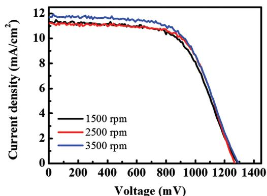
**Figure 3.** LIV results of tandem solar cells with different spin coating conditions of PCBM layers.
