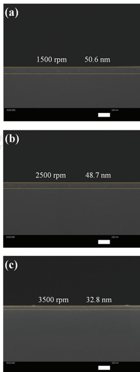
**Figure 4.** SEM images of PCBM layers with different spin-coating condition (a) 1500, (b) 2500 and (c) 3500 rpm.
