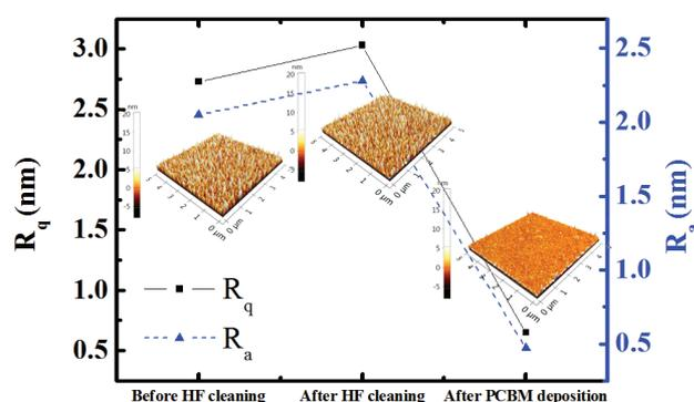
**Figure 1.** Root mean square and average roughness of surface according to the sequence of PCBM deposition with AFM images.
