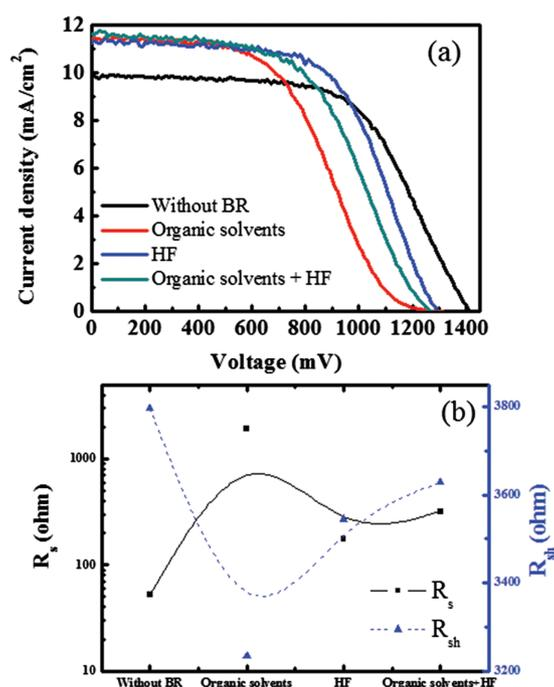
**Figure 2.** (a) LIV results of tandem solar cells with different interface treatment conditions between  $n\text{-}\mu\text{c-Si:H}$  and PCBM layers and (b) sheet resistance and shunt resistance of the cells.
